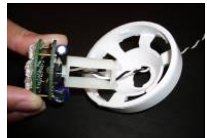
Bayonet Mount in Lens Base
